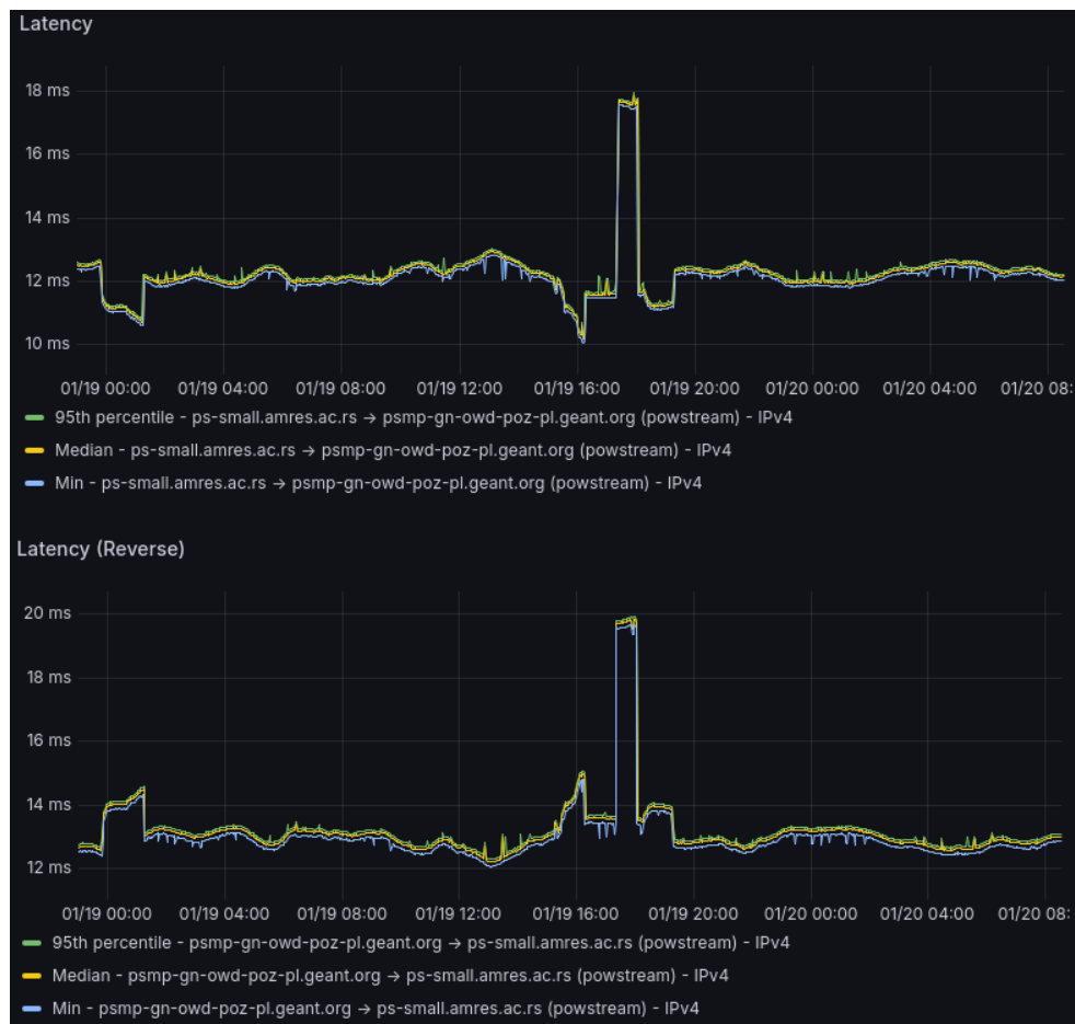
Figure 5.2 Reconstruction OWD latency measurements, where only minor fluctuations are visible
