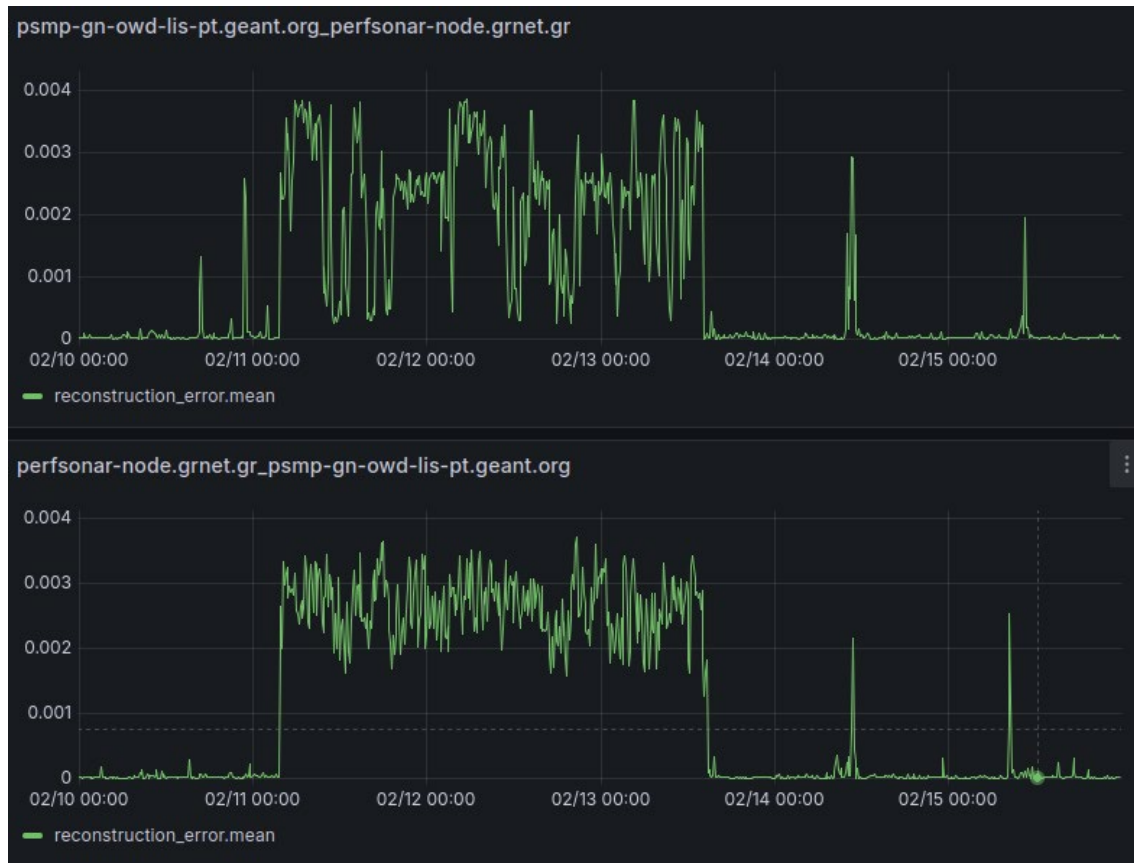
Figure 5.4 Reconstruction error for both measurement directions between two perfSONAR nodes. Prolonged anomalous event is observed
