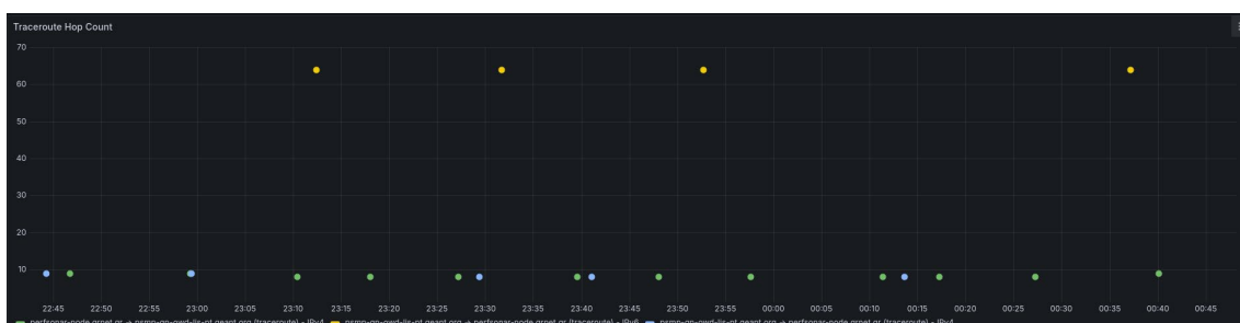
Figure 5.8 Traceroute hop-count variation during the same interval as the sustained anomaly, showing a reduction in the number of hops
