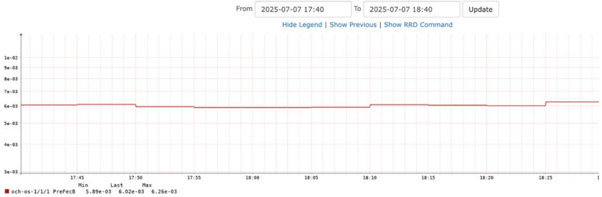
Figure 4.20: Pre-FEC BER on the first wavelength at the Vienna end of the link
