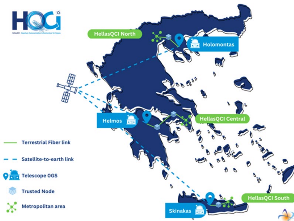
Figure 3.1: HellasQCI project network topology
