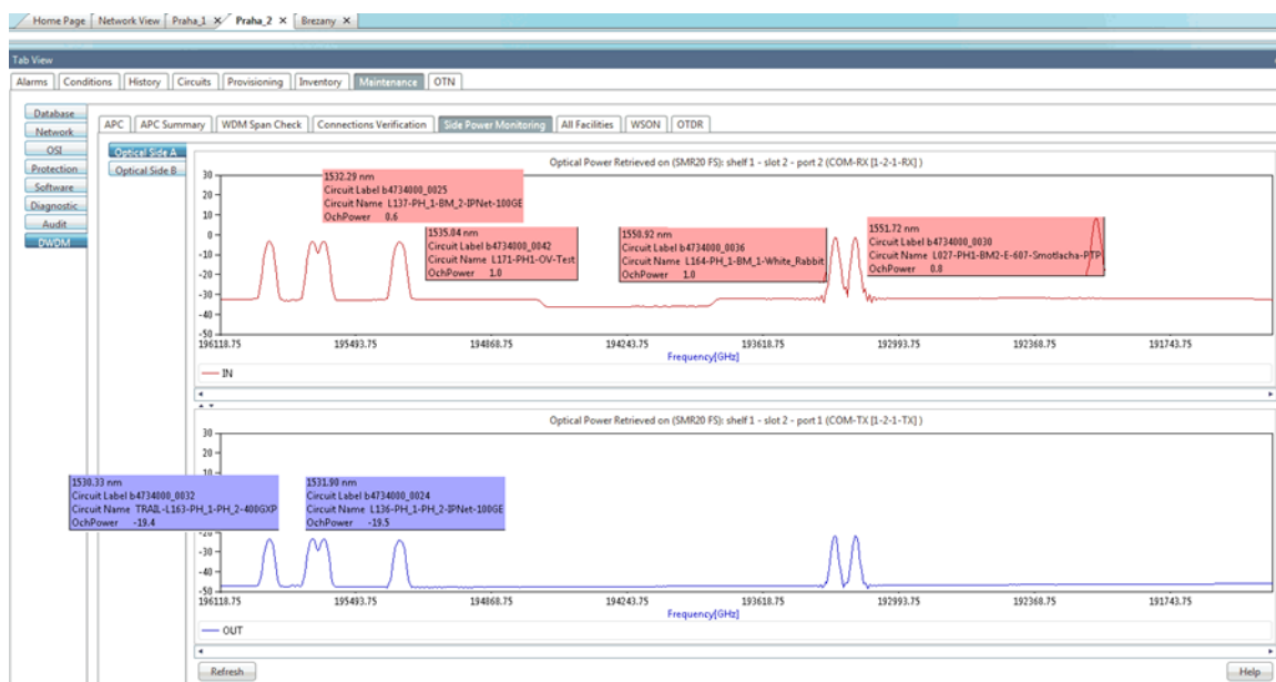
Figure 5.11: Spectral plot from Cisco NCS system showing parallel transmission of coherent 400G lambdas and WR signals within the DWDM
