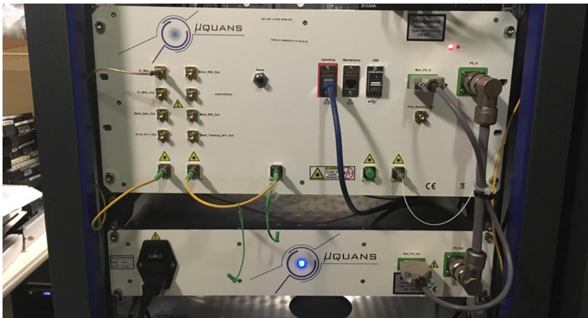
Figure 4.3: Repeater Laser Station connected directly to the routers (blue Ethernet cable) in an extremity site
