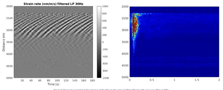
Figure 5: Strain rate recorded at the entrance of the fibre in the water (2.25km) filtered with a low-pass filter at 30Hz. The shallow water ends after around 4.5km of cable. Right: Frequency content of strain rate signal along the fibre
