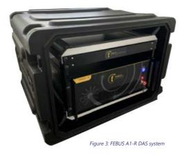
FEBUS OPTICS is an innovative company based in Pau (France), that brings a new generation of optical fibre-based sensor system to the market, for the maintenance and monitoring of infrastructures. Its patented technology uses state-of-the-art optical physics to measure temperature, strain and vibrations of a structure or soil over tens of kilometres. FEBUS manufactures DAS, DSS, and DTS equipment, and provides high performance equipment, solutions, and its expertise to a wide variety of markets.
