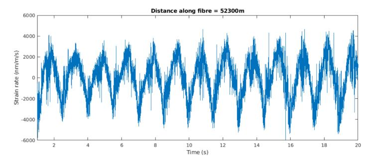
Figure 6: Top left: Strain rate along the end of the fibre (from 50km to 56.5km) filtered with a low-pass filter at 30Hz. Top right: Frequency content of strain rate signal at the same distance. Bottom: Strain rate signal at 52,300m in nm/m/s
