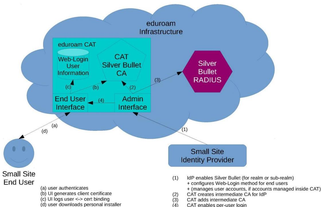
Figure 3.1: IdP-as-a-Service solution architecture
